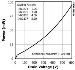
Figure 31. Drain Capacitance Power.
