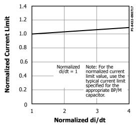
Figure 32. Standard Current Limit vs. di/dt.
