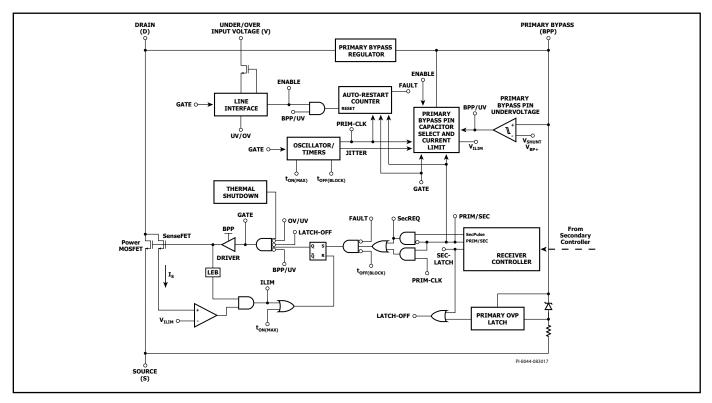
Figure 4. Primary Controller Block Diagram.
