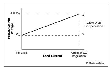
Figure 9. Cable Drop Compensation Characteristics.
