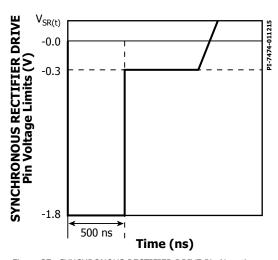
Figure 27. SYNCHRONOUS RECTIFIER DRIVE Pin Negative Voltage.
