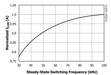
Figure 7. Normalized Primary Current vs. Frequency.
