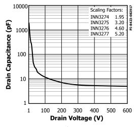
Figure 30.  $C_{\rm oss}$  vs. Drain Voltage.
