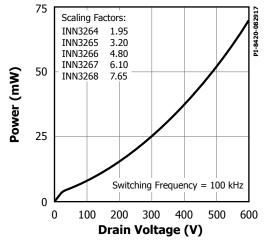
Figure 25. Drain Capacitance Power.
