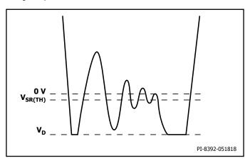
Figure 13. Unacceptable FORWARD Pin Waveform After Handshake with SR MOSFET Conduction During Flyback Cycle.
