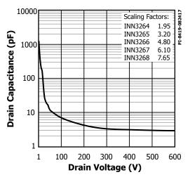
Figure 24.  $C_{OSS}$  vs. Drain Voltage.
