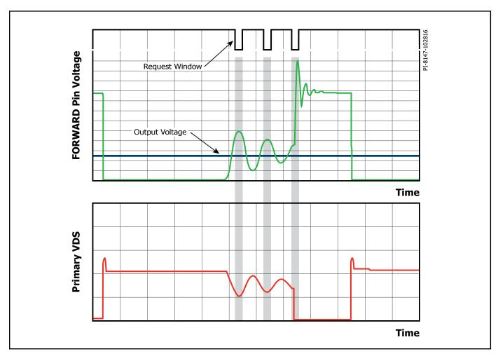
Figure 10. Intelligent Quasi-Resonant Mode Switching.
