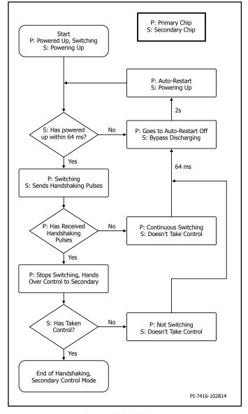
Figure 8. Primary-Secondary Handshake Flowchart.
