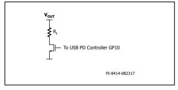
Figure 12. Active Pre-Load Circuit.
