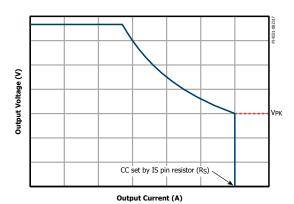
Figure 3. Typical Constant Power Characteristics.
