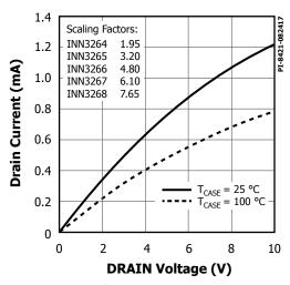
Figure 23. Output Characteristics.
