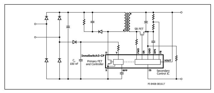
Figure 18. Fast AC Reset Configuration.
