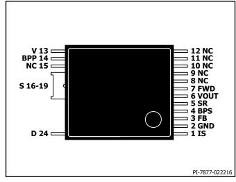
Figure 6. Pin Configuration.
