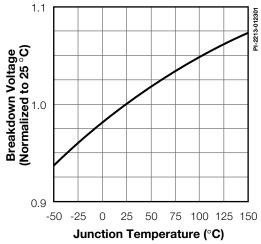
Figure 26 Breakdown vs. Temperature.
