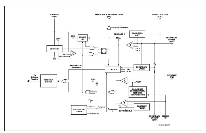
Figure 5. Secondary Controller Block Diagram.
